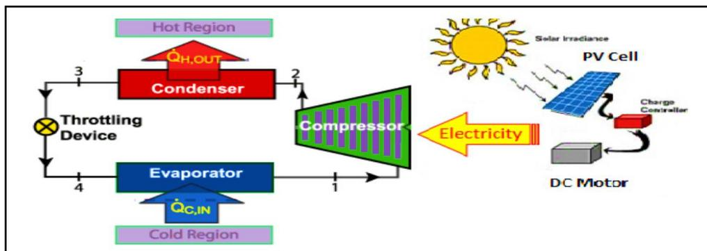
Fig. 6. Photovoltaic Operated Refrigeration Cycle [10].
