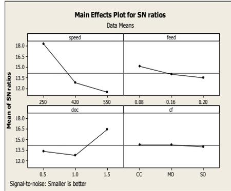
Fig. 1. Effects of the S/N Ratio on Tool wear.
