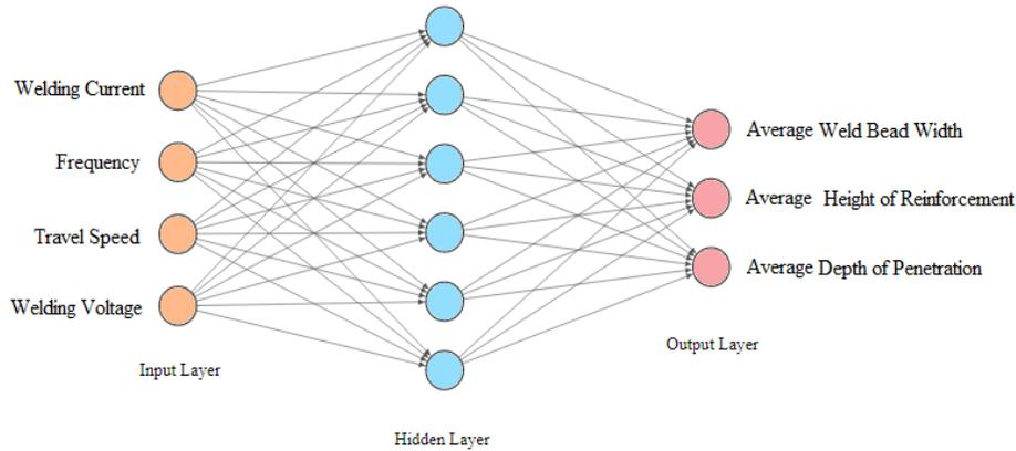
Fig. 3. Schematic Diagram of ANN Model for predicting Bead Geometry.
