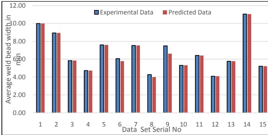
Fig. 10. Comparison between experimental and predicted data of weld bead width.
