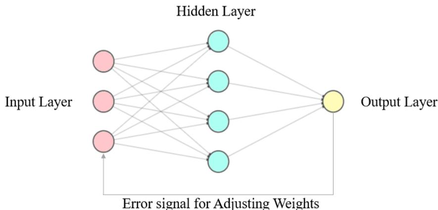
**Fig. 2.** A Typical Back Propagation Neural Network Model.
