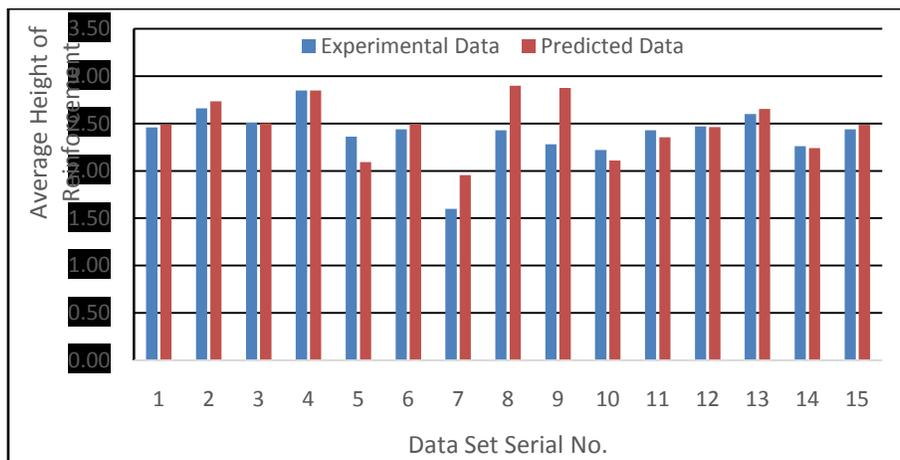
Fig. 9. Comparison between experimental and predicted data of height of reinforcement.
